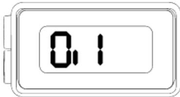
The 'Oil' odometer will display the distance travelled since the last oil change. Its value can therefore be reset by holding the '-' key.
