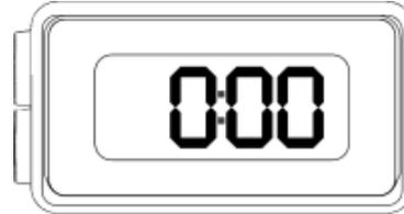
To adjust the time, press and hold the '-' key whilst in clock mode. The flashing digit can be incremented with the '+' key, toggling between minutes and hours is done by the '-' key.
