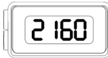
Clicking the '+' key allows to increment the currently selected digit that is flashing. The selected digit can be changed by holding the '-' key.
